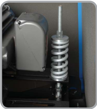
Automatic V-belt drive tensioning system
